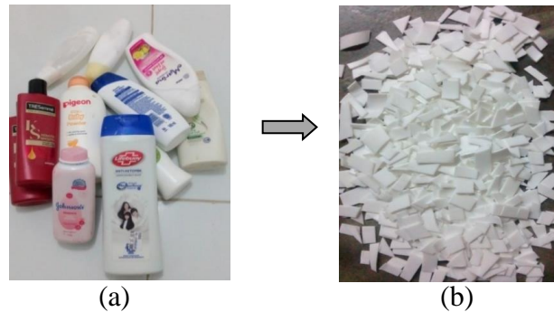
Figure 1 (a) HDPE waste and (b) HDPE waste after cutting
