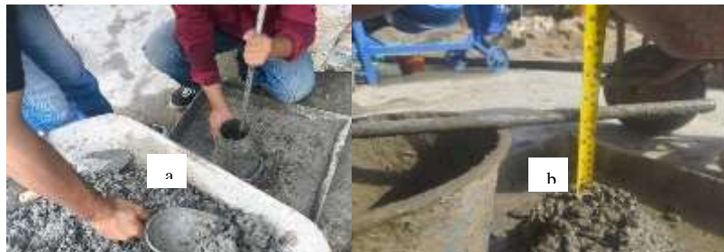
Gambar 1 Pengujian Slump (a) Proses Uji Slump (b)
